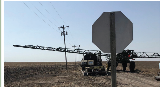
A Kansas farmer dangerously parks a self-propelled sprayer directly under a power line.
